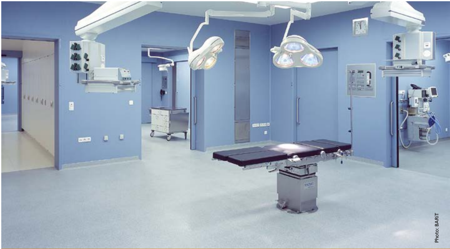
BARiT ATEX-TERRAZZO, electrically conductive | Clean Room Floor | Kinderklinik Aschau
